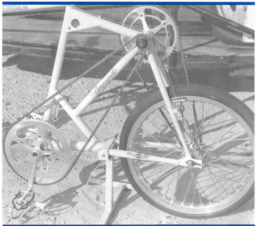
SPEED ATTEMPT - A Close-up look at the HUJSK Double Reduction Drive System
