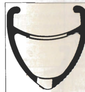
Section of aerodynamic rims
