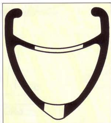
Section of aerodynamic rims
