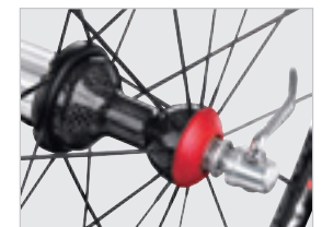
Rear hub in structural carbon with variable thickness, with titanium pawl carrier and ceramic spheres
