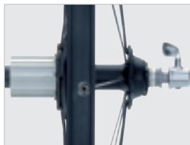
Asymmetrical rear wheel for better dish balancing
